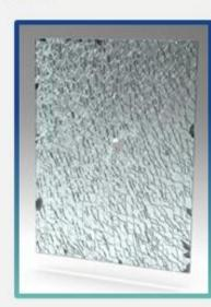
Resistant to breakage, 4x as strong as annealed glass, shatters completely in small pieces, typically vacates the frame after impact.
