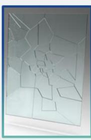
Resistant to penetration, breaks upon impact, tends to keep shards intact upon and after breakage. Two or more pieces of glass adhered together by interlayer.
