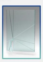
Resistant to breakage, 2x as strong as annealed glass, breaks in large shards.
